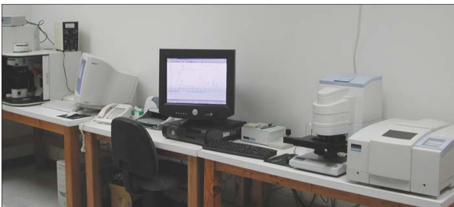
Figure 1. PerkinElmer Spectrum One FT-IR System and the AutoIMAGE microscope in the Microtrace laboratory.
